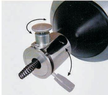
Cable rotation adjusted by pressing wheel. Cable feeding and relative speed controlled by drive handle.
